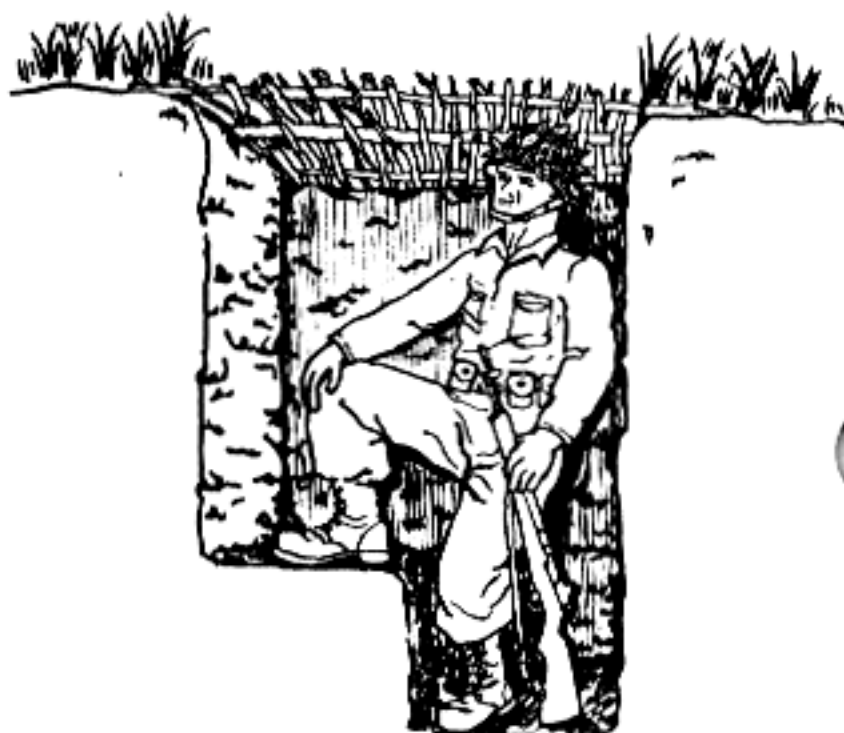
Figure 27. Details of a foxhole cover.
